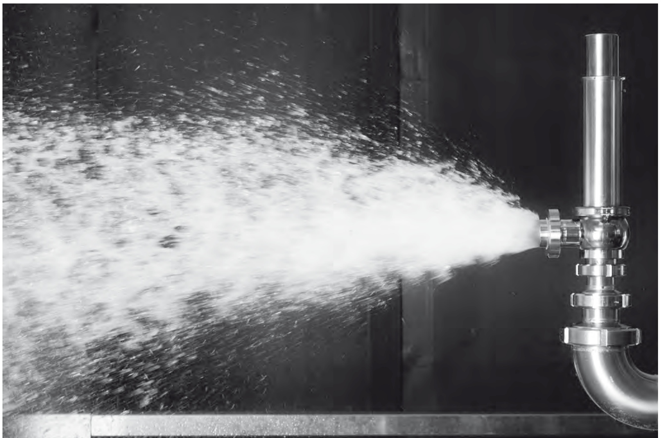
Safety valve in the Guth Ventile test centre
